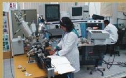
Scanning Auger Microprobe
