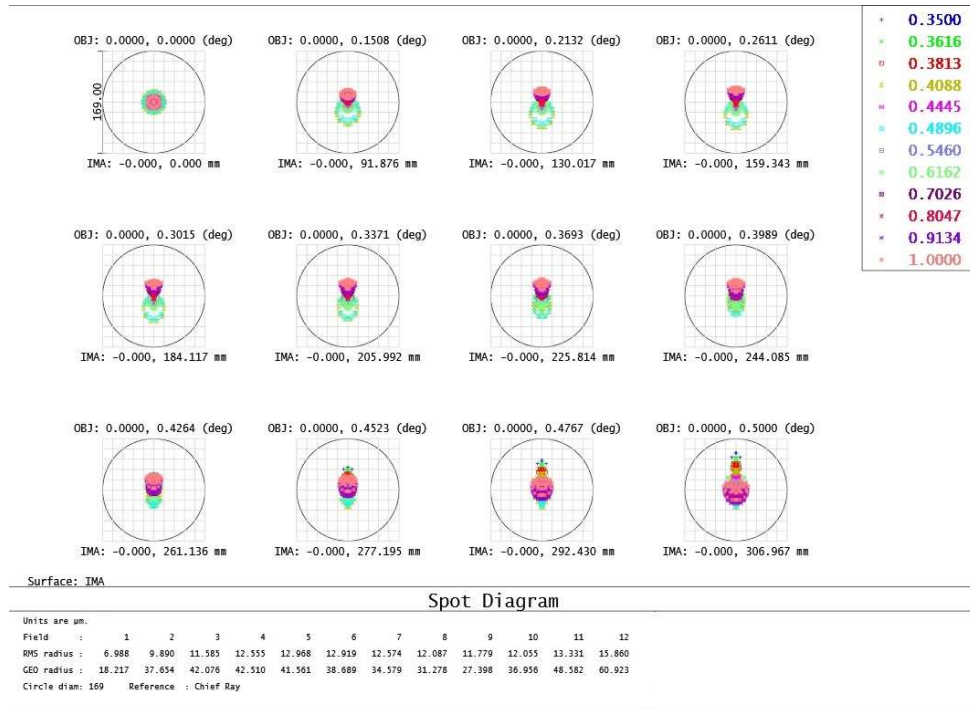
Figure 17. Imaging mode spot diagram, the circle corresponds to 1".
